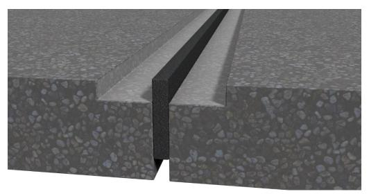
Place foam blockout in joint opening.
