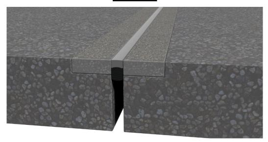
Install TuffSeal SL-1 or other desired sealant.
