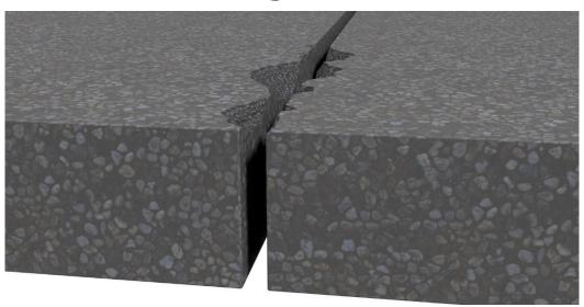
Layout and mark joint blockout: 4" minimum to either side of the joint or 6" if joint opening or movement is greater than 1".
