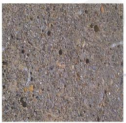
Fig #1 Pinholes in concrete
